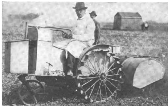
Left—La Motoculture machine with driver astride four-cycle motor. Right—Bull tractor in Grigny demonstration
